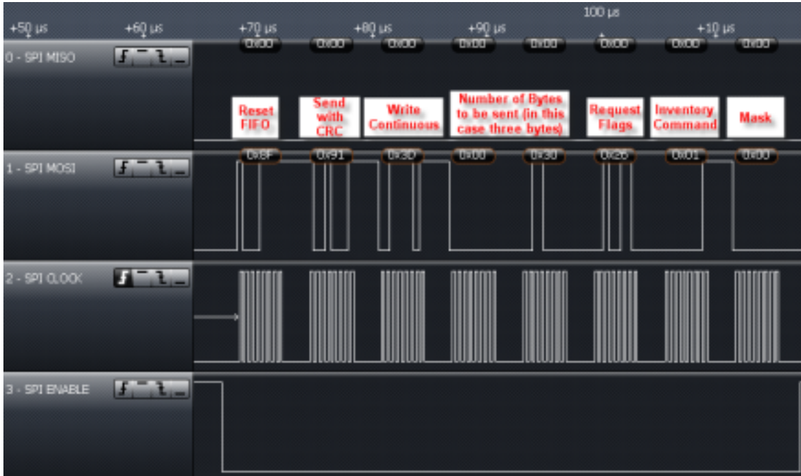
Figure 5-20. Inventory Command Sent From MCU to TRF7964A
