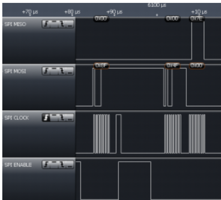
Figure 5-25. Reset FIFO and Read RSSI
